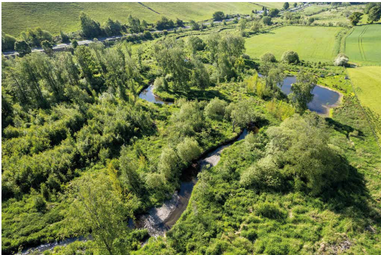
Figure 2. Lake Wood remeander reach 10 years after creation, showing development of in-channel sediment bars and riparian woodland. Photo credit: Colin McLean.
