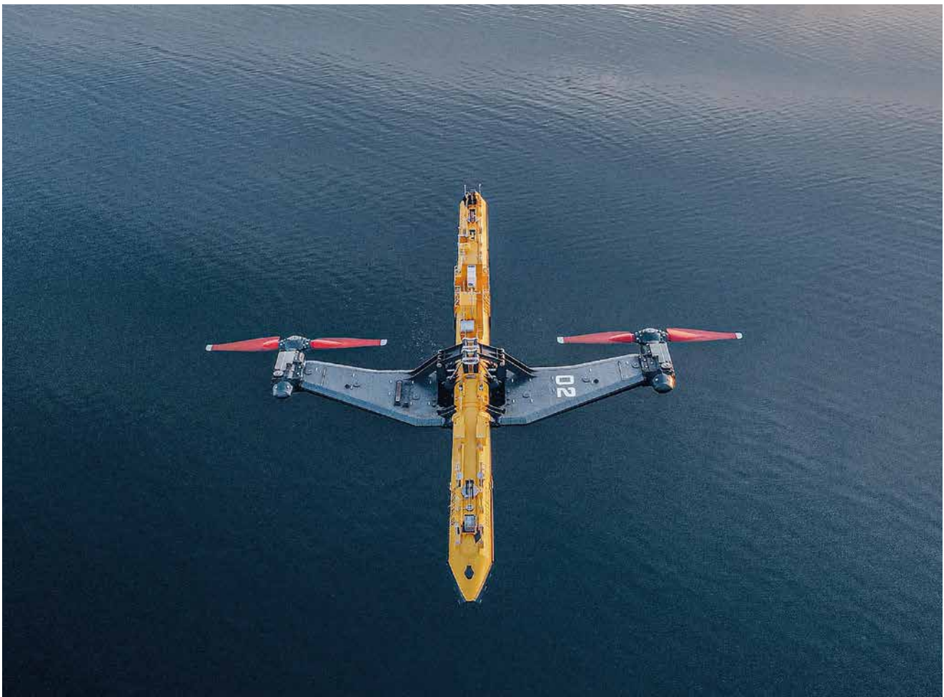
Figure 2. Orbital Marine Power (OMP) uses floating tidal technology. Reproduced under the Creative Commons Attribution-ShareAlike 4.0 licence.
