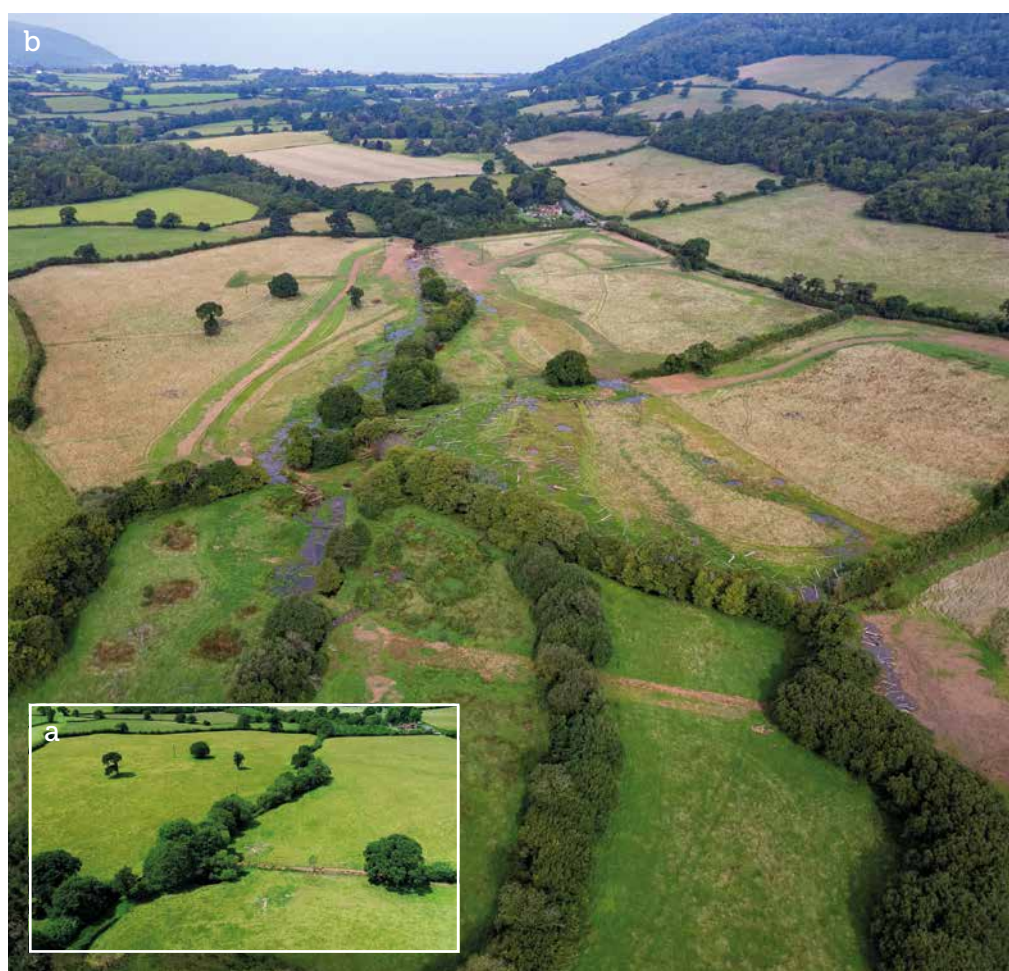
Figure 3. River Aller, Somerset, Stage 0 restoration, where a 1.2 km straightened and deepened section of the river has been in-filled to reconnect the river and floodplain. (a) Pre-restoration river 'hidden' in the central hedge line; (b) immediately post-restoration (September 2023) the river found new routes across the floodplain and created 7 ha of multi-channel wetland. Woody material (4000 tonnes) was added to increase habitat complexity and surface roughness and over 25,000 trees and wetland plants were planted. The site has continued to develop since, with additional complexity of channels, numerous ponds and pools, an increase in groundwater levels and an abundance of wildlife. Photo credit: National Trust & View It 360.
