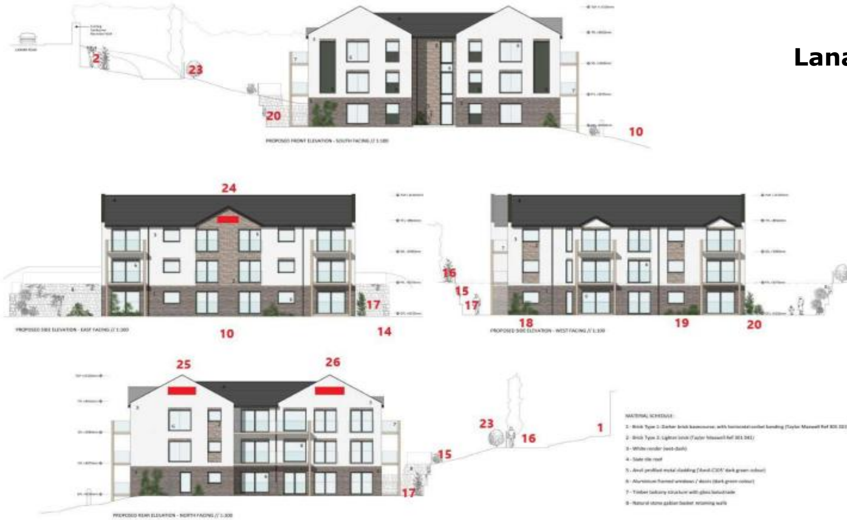
Figure 6 Elevations showing locations of biodiversity enhancements, including integrated swift nesting blocks on Eastern and Northern elevations
