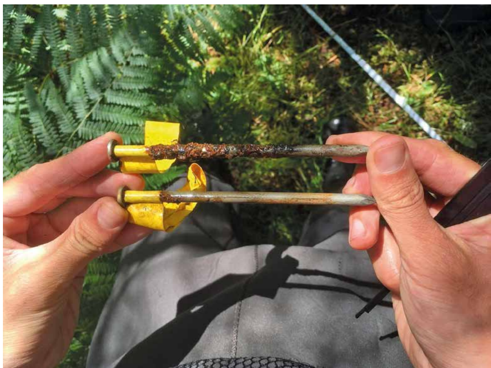
Figure 2. Ungalvanised nails (12.5 cm) that had been hammered into the riverbed substrate to 10.5 cm depth and left for 4–6 weeks. The uppermost nail had been placed in oxygen-rich riverbed substrates and is heavily encrusted. Photo credit: Kieran Leigh-Moy.
