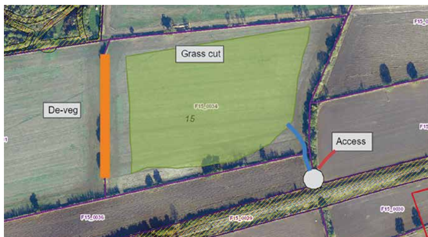
Figure 3. An example of a small manageable area covered by the Fusion Ecology and Arboricultural Permit (EAP) process for vegetation management activity in a single field and adjacent hedgerow. Map shows an area of proposed grass cutting (green) and hedgerow removal (orange) and the clearance contractor’s proposed access route (blue).
