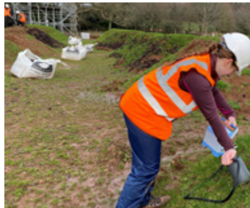
IRGA analysis for soil CO 2 efflux - Mark Nason
