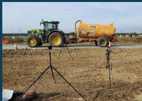
Noise measurement of dust suppression bowser
