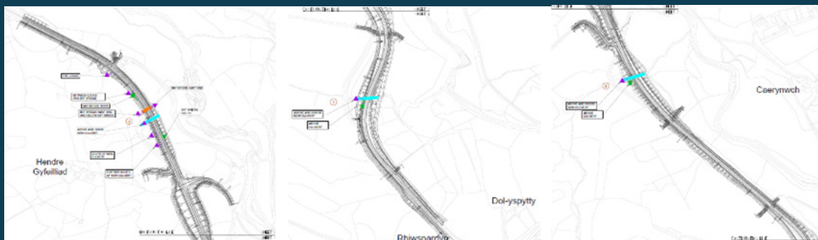
Diagrams show the distribution of the oversized culverts (2.7 m diameter) along the scheme (blue bars).
