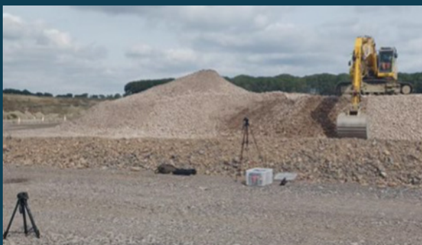
Noise measurement of stockpile management
