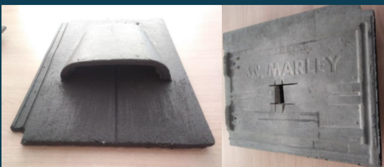
Marley custom-built concrete bat access tile with a baffle covering the bat access gap and a roughened surface to the front for enhanced grip; and rear view of bat access gap.
