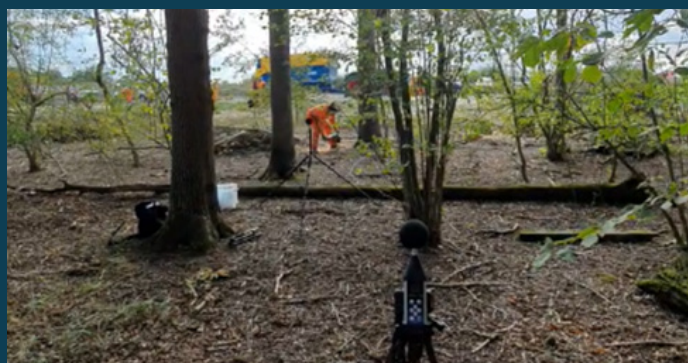
Noise measurement of chainsaw tree felling
