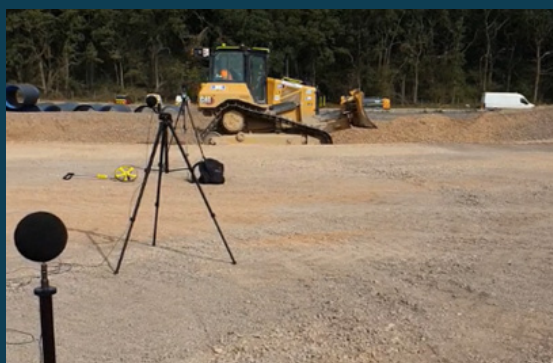
Noise measurement of dozer in action
