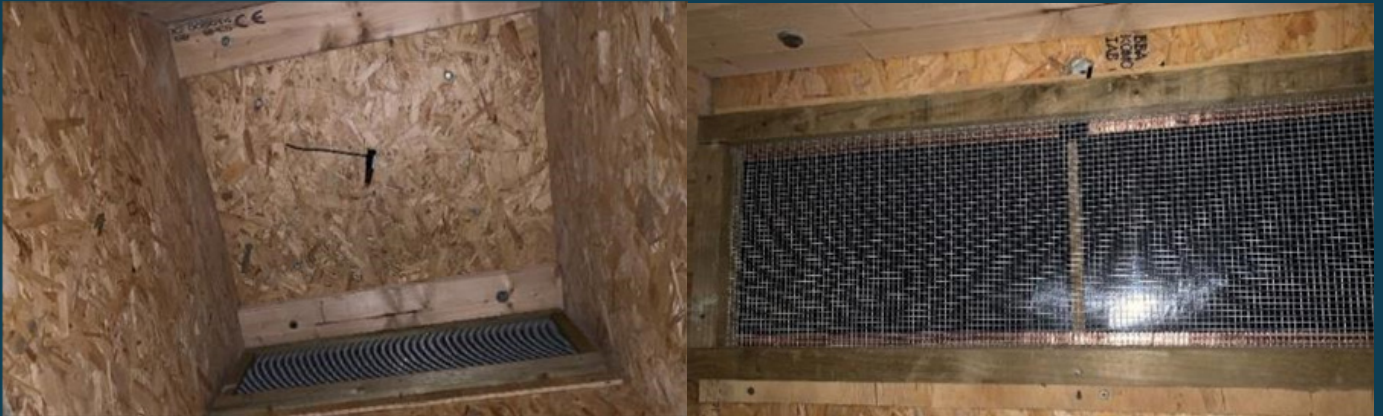
Heated hot box: infra-red heat matting provides heat from one side, offering a heat gradient across the box. The heating is powered from a nearby lighting column and the South-West Trunk Road Agency maintain/check that the power is on as part of their routine inspections.
