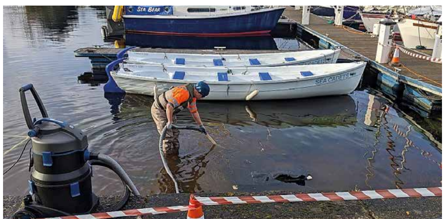
Figure 3. Use of a pond vacuum in an aquatic survey area. Photo: Ecus.
