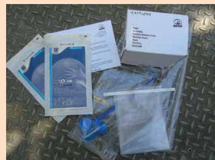
Figure 2. eDNA sample collection kit comprises the following sterile equipment: a plastic scoop/dipper, two pairs of gloves, a transfer pipette, and 6 tubes containing preservative within a small box.
