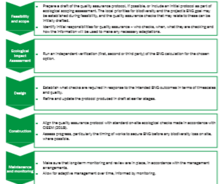
Figure 5.1 Key actions for quality assurance of the implementation of biodiversity net gain through the project life cycle
