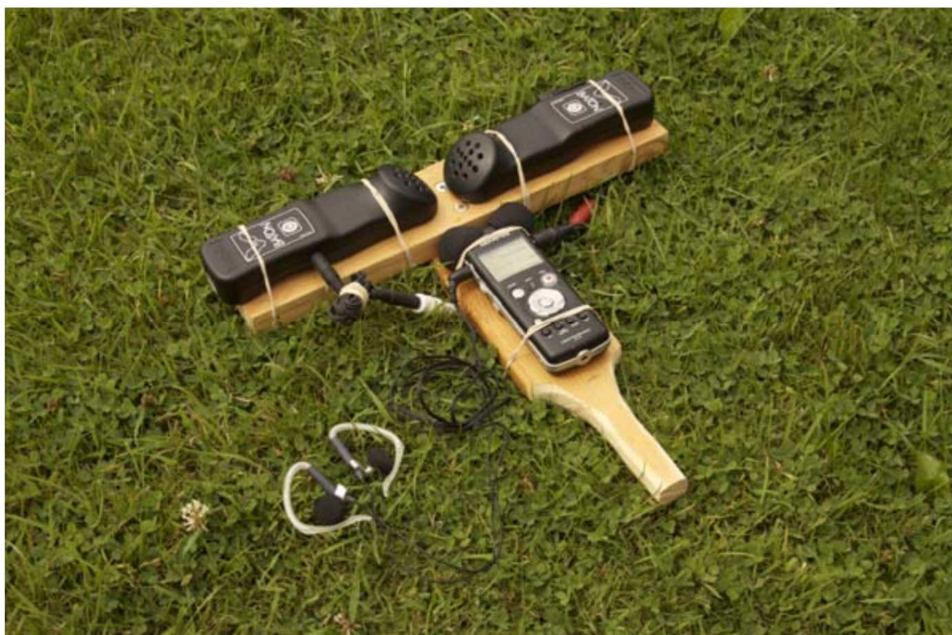
Figure 9. A simple Batstick setup to listen, in stereo, to bats during hand-held surveys
