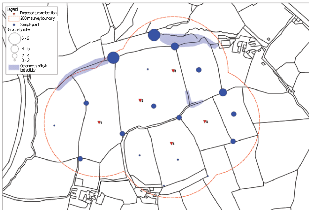
Figure 1: Example of a bat activity summary map for a hypothetical proposed wind farm site. Bat pass rates are shown for each sample point as blue circles (size indicates mean bat passes per five minute sample period). This data can be grouped into the three species risk categories (Low, Medium and High) suggested by Natural England and presented on separate maps. Other areas of high bat activity are shaded blue. These areas can be identified by plotting all non-sample point bat records on a draft site map.
