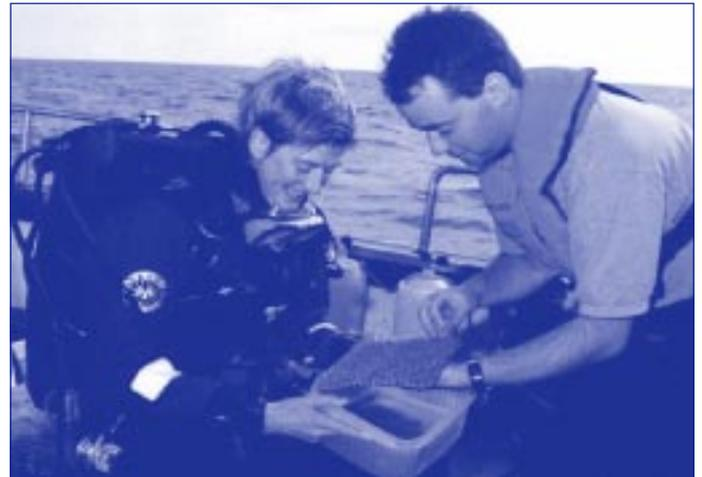
**Figure 7. Carpet tile recovery for sediment load measurement**
